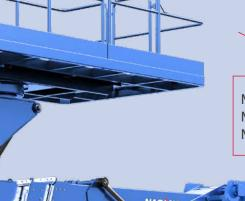
Max platform height: 9 m Max working height: 11 m Max moveable load: 600 kg
