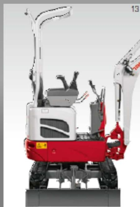
PORTE-A-FAUX MINI A L'ARRIERE AVEC UN TRAIN DE CHAÎNE DE 1.020 MM LARGE
