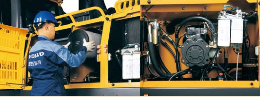
• Simplified, ground level service access.
