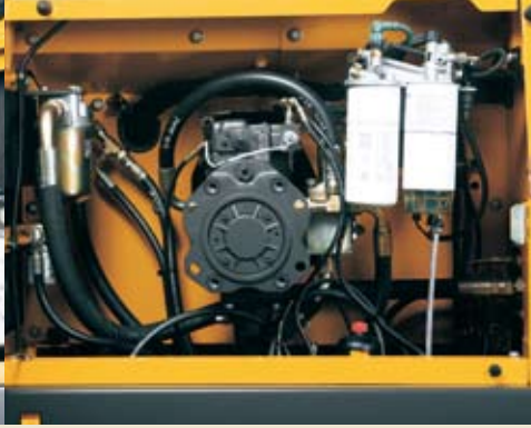
• Easy access to hydraulic pumps and filters.
