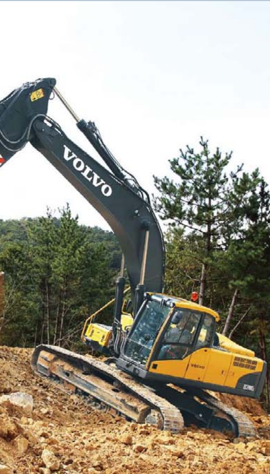
• Lifetime greased sealed track link.
