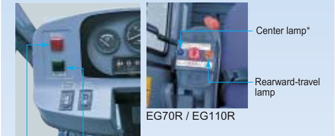
EG40R * Lit when the upper structure and undercarriage become paralleled.
