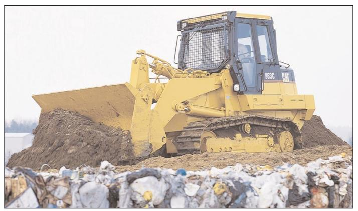
Waste handling/demolition attachments provide added versatility and are designed to make the 963C perform well in sanitary landfills, waste handling or demolition applications where the machine spreads, compacts, sorts, shreds and crushes materials.
