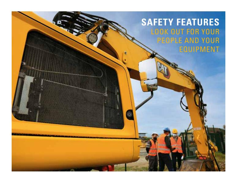
Daily maintenance checks can be performed with 100% of the points accessible from ground level, making maintenance faster, easier, and safer. Standard LED lights give you a better view of your jobsite.
