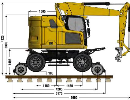
All dimensions are approximate and may vary depending on front linkage position or tires for ground clearance.
